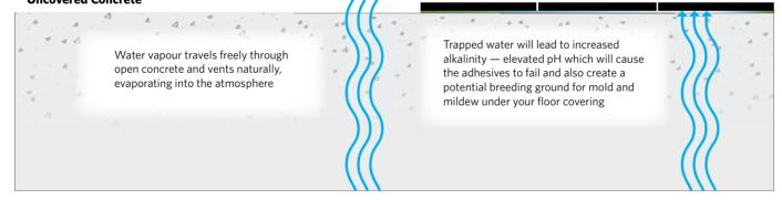
**Water can cause all kinds of problems.** Moisture seeks equilibrium. It essentially just wants to evaporate. Water vapour will naturally rise until something gets in its way. Concrete is filled with vertical capillaries and does not hinder the process.
